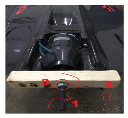
5. Take a blade and slide it between jet pump housing and board housing, thus cutting out any sealant. After that, try to pull out jetpump, it will not be easy. Be careful.
